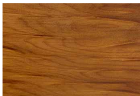
KAURI "LEVIGATO", OLIO Kauri "machine sanded", oil Kauri "geschliffen", geölt
